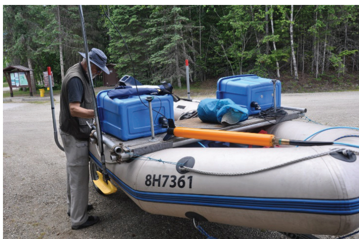
Figure 5. Harry Bohm with the Marine Magnetics towed magnetometer and pole-mounted Starfish side scan sonar in a Mercury 4.3 m inflatable (Pollack 2020).
